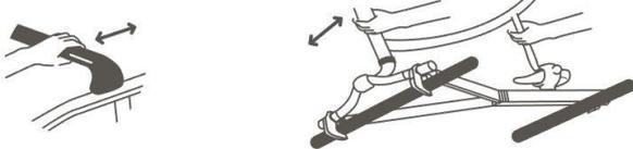
Check cross rails cannot move after bike and rack are installed. Check bike cannot move across the cross rails.
