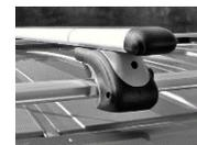
Bolt or secure ISO approved clamp to longitudinal rails
